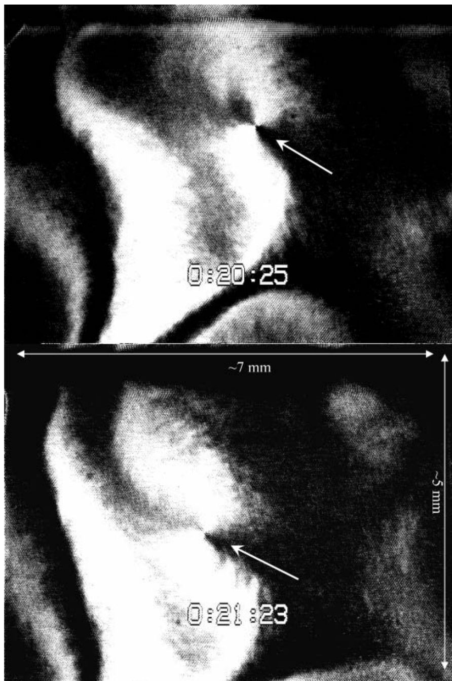
Figure 6. An example of a set of images used to calculate the speed of a point defect in a 2M4P9OBC free-standing film. The two successive images were digitally captured from a DRLM videotape with the tape counter displayed on the screen. In the roughly one minute between images, the point defect (indicated by the diagonal white arrows) moved down and slightly to the left. The defect drifted nearly in a straight line, with a slight curvature in the clockwise direction. The approximate dimensions of the frames are shown.
